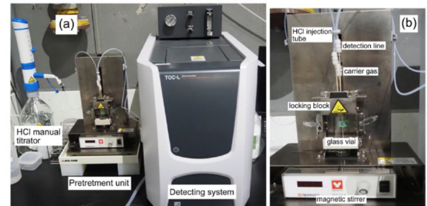
Fig. 1. AD-TIC measurement system, (a) Overview, (b) Pretreatment unit.
